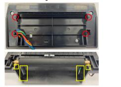
5. Reassemble the Cover Roller L&R that was removed in step 2.
