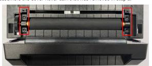
Place the bottom of the Printer face the front. Insert the Auto Cutter Wire into the Auto Cutter Connector(red square) in the correct direction.
